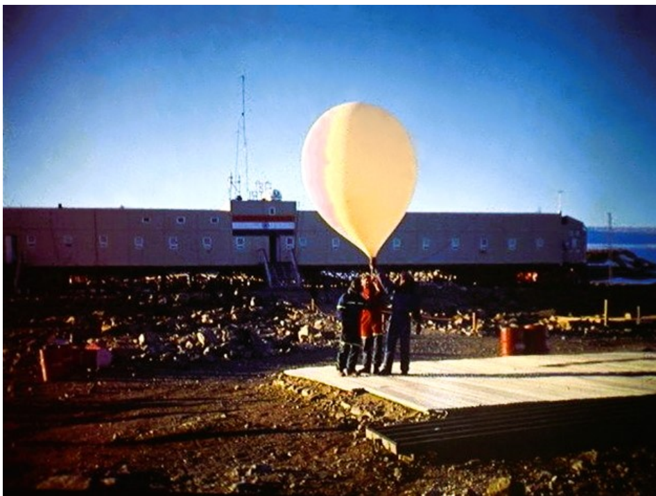
Ballooning experiment by IMD to assess the upper atmospheric condition
