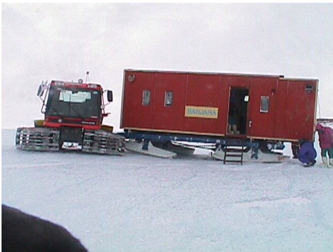
The convoy carries a living module called 'Banjara', and a fuel generator named 'Jeevan Jyoti' with fuel tank with 5KL. Banjara is heated from inside and is equipped with a small kitchen and bio-toilet.
