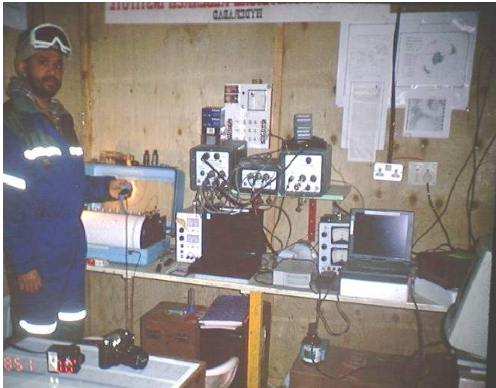
Seismological observatory at Maitri, Antarctica, featuring analog and digital seismographs. The author demonstrates static body discharge using a wristband-the first assignment.
