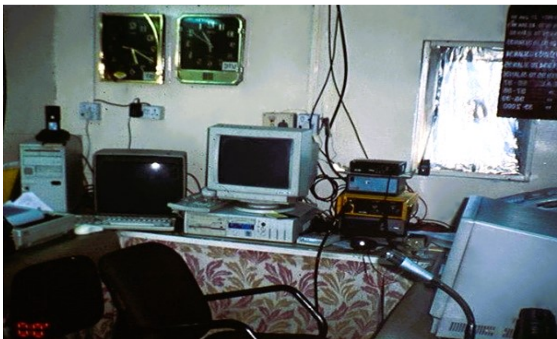
Communication hub at Maitri Station, featuring a range of equipment including satellite phones, HF communication, loudspeaker and a FAX machine. The clock displays the time difference between Antarctica and India.
