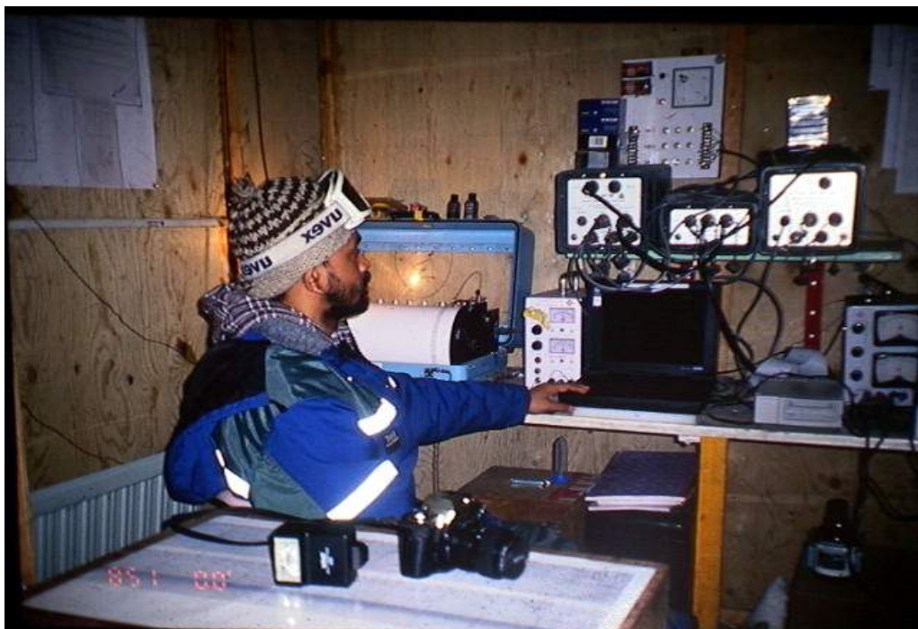
Interior of the seismological observatory showcasing the sophisticated digital setup for earthquake monitoring. An oil heater (left) maintains room temperature around 5°C. Heat-sensitive white chart paper captures analog seismograms, while a digitizer records and displays signals as digital seismograms on a laptop computer for further analysis
